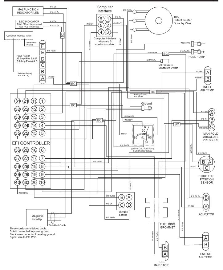
Figure 32. EFI Wiring Diagram
